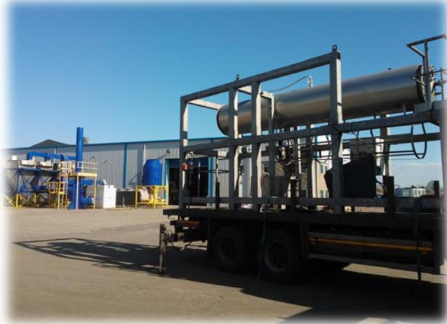
*Photo on left shows pre-commercial scale wastewater treatment technology (on truck-bed) developed by TCBB & NUI Galway with NVP Energy—produces biogas; also, Premier Green Energy's advanced pyrolysis technology (located on the site of the former Thurles sugar factory) is in the background*
