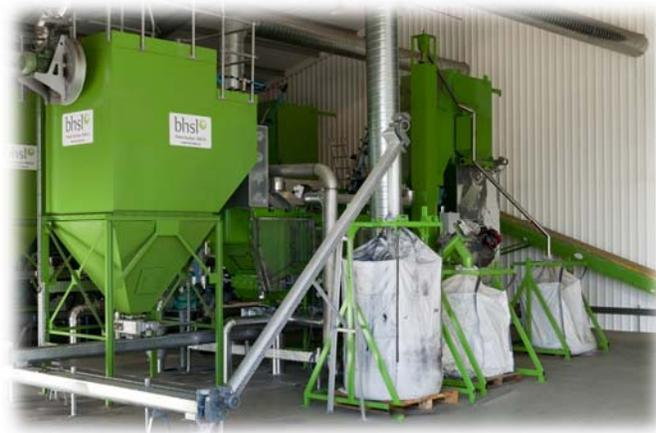
**Fluidised bed combustion technology for heat and electricity by Irish company bhsi - bioenergy from poultry manure for poultry farms.**
